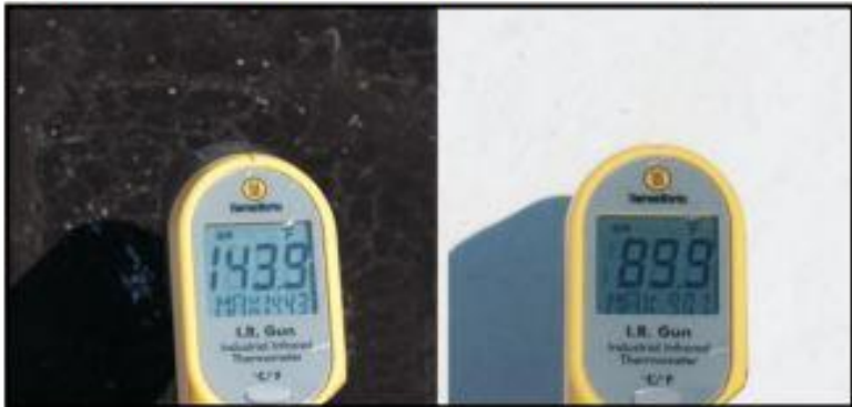
Figure 1: Dark vs. Cool Roof Surface Temperatures
